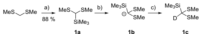
Scheme 2. (a) n -BuLi (1.1 equiv), Me 3 SiCl (2.0 equiv), THF, –70 to 0 °C, overnight; (b) n -BuLi (1.1 equiv), THF, 30 min at –78 °C, then 30 min at 0 °C, finally 15 min at room temp; (c) D 2 O.
